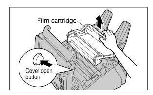
**1** If the film is slack, tighten it by winding the gears.
